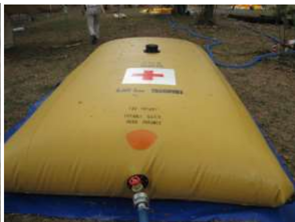
Figure 1.3: Bladder Tank 5,000L Capacity
