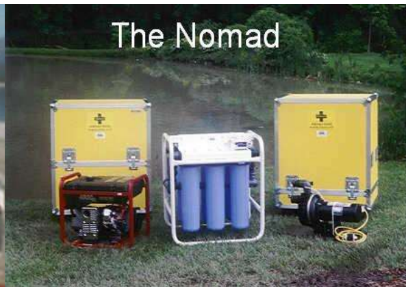
Figure 1.5: NOMAD treatment plant
